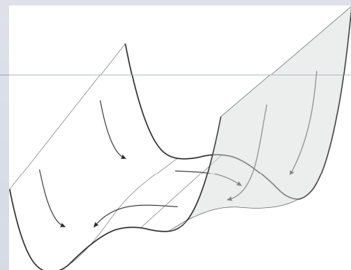
Fig. 4. Hypothetical flow field reconstructed from the flow directions in the phase plot. In case of harmonic oscillator, such field corresponds to potential with quadratic curvature near its minima.
